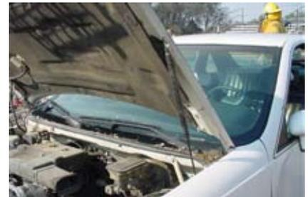
*Even small hood struts like the one shown can violently and unexpectedly explode during a fire sending an arrow like projectile through the air.*
