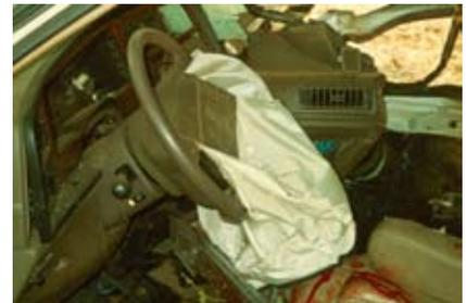
*Air bags are hidden in the steering wheel, dashboard, upholstery, and can deploy from the roof or pillars of the vehicle.*
