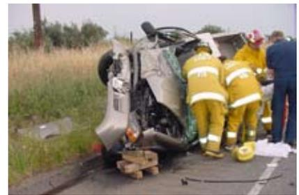
*Stabilizing the vehicle is essential to safe rescue operations.*
