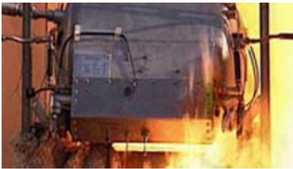
*This Hydrogen cylinder is undergoing the bonfire test.*
