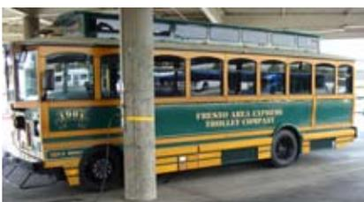
*Natural gas mass transit vehicles are easy to identify with their characteristic hump on the roof, where the CNG cylinders are stored.*
