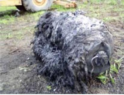
*A vehicle fire and inoperative pressure relief device (PRD), allowed this cylinder to fail.*
