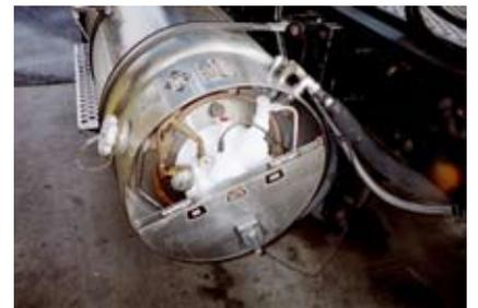
*Ice crystals around the LNG tank valves during re-fueling is normal.*
