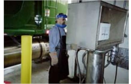
*LNG re-fueling is handled by skilled professionals. Note the Protective gear, rubber apron, gloves, and face shield to protect the operator from cryogenic burns.*
