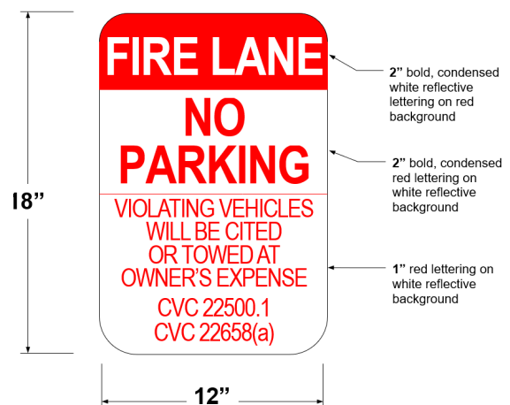
Figure 5 – Fire Lane No Parking Signs
